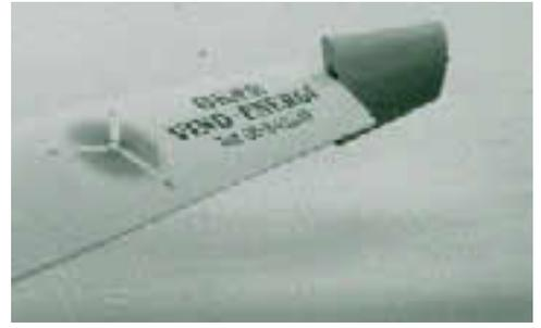
May 1978 the first set of 5 m blades were delivered and later that year they were supplied with revolving tip brakes. This blade soon became standard on several types of wind turbines. Once more the inspiration came from Juul's Gedser turbine.
