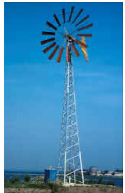
**Among the heat-producing wind turbines, the "SJ-Windpower" was popular, combining traditional windmill technology with modern materials. And the users avoided problems with coupling to the public grid.**
